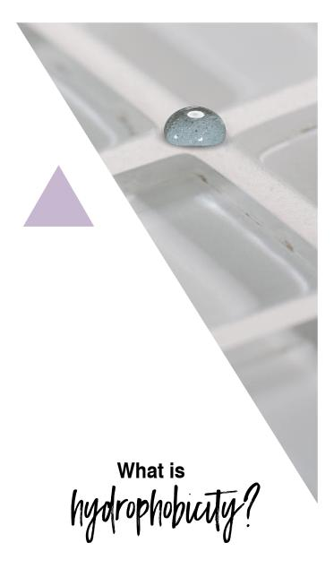
**Hydrophobicity** is the ability of the molecules of a given material to repel water. In the case of grout, this means that water cannot penetrate into the joints - water drops roll off the surface of the joint.
