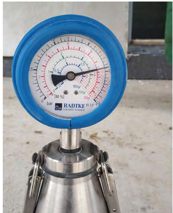
SCREED MOISTURE CHECK
